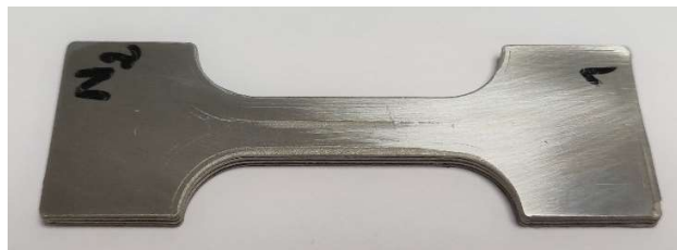
Figure 35: Sintered and polished tensile specimen
