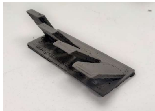
Figure 30: Test part of the printable inclination without support (30°, 40°, 50°, 60°) (green part)
